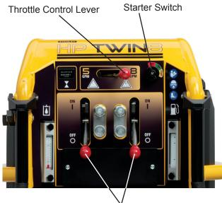
Flow Control Lever(s) In Off Position
